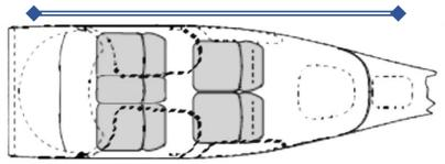
**5 Seat Configuration**: 2 Crew Seats and 1 Rear Bench Seating (1 standard + 1 expanded to accommodate a small child)
