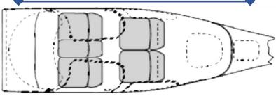
**5 Seat Configuration**: 2 Crew Seats and 1 Rear Bench Seating (1 standard + 1 expanded to accommodate a small child)
